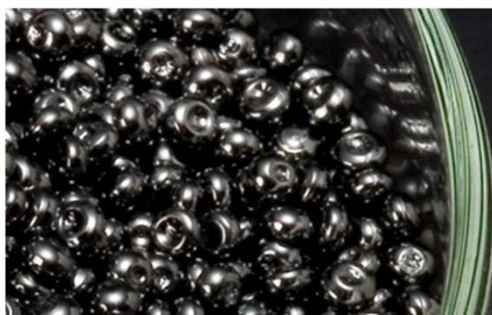
Standard granule size 2.0 – 3.5mm
