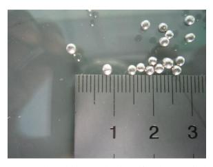
\* In granules will be supplied in uniformly controlled globular shape with about 2mm to 3mm diameter.
