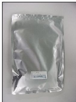
Inner Al bag purged with N2 gas
